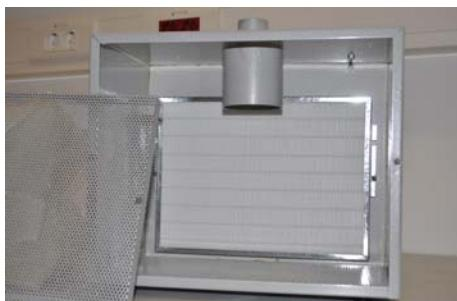
1. Loosen the two knurled nuts on the maintenance cover.
