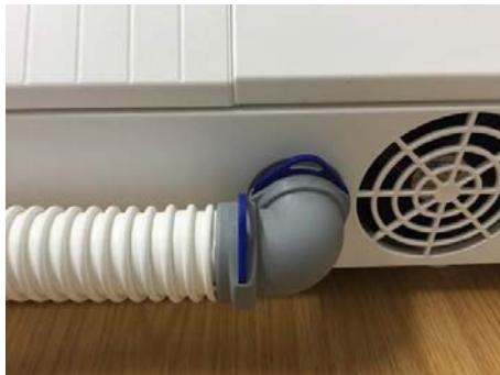
1. Connect one end of the suction tube to the available connection point on the suction device. The connection point is located on the top side next to the control panel with the suction power controller.
